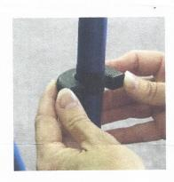
Hold the UniClamp (Fits tubes from 3/4" to 1 3/8" dia and some square tubes.) to the tube where convenience item is to be mounted.
