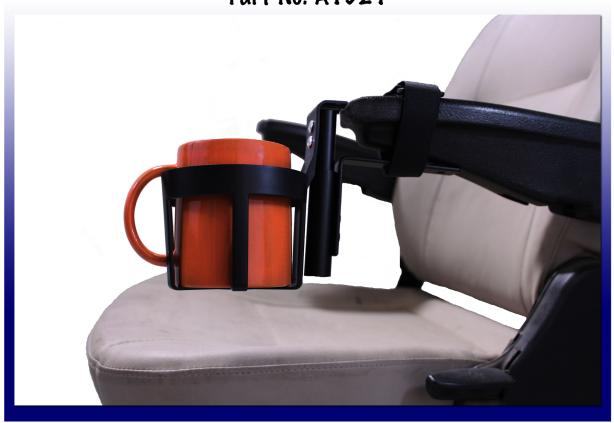
When there is no accessible hardware, the hook and loop strapping system will allow you to mount a cupholder to the end of any armrest.
